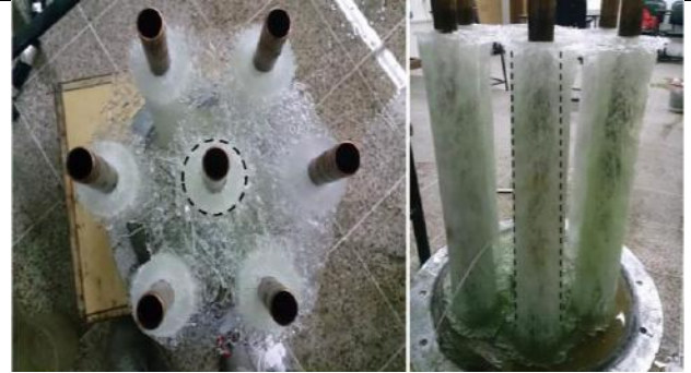
Fig.14: Actual ice thickness in the storage tank.
