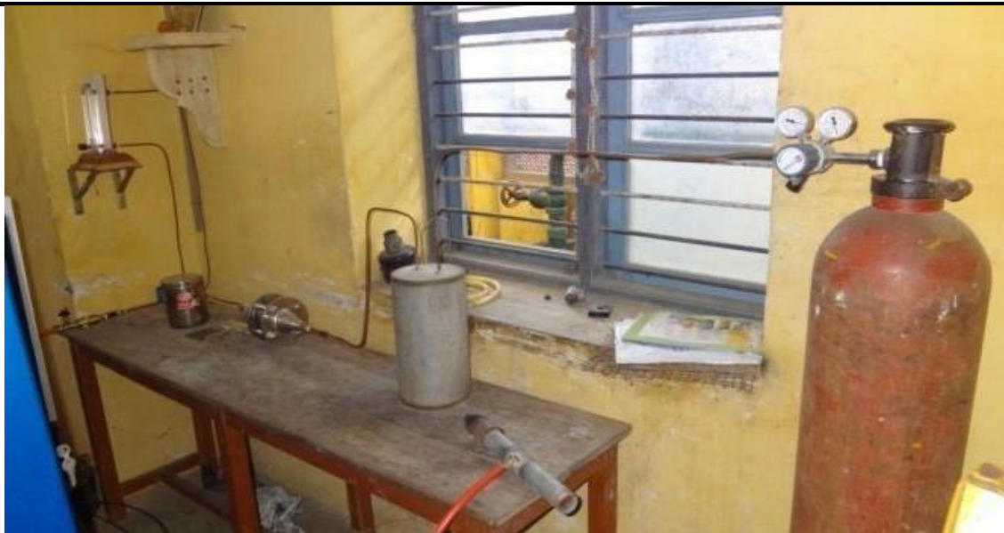
Fig.3: Hydrogen Gas Induction Set up
